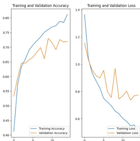
Figure 2. Resulting graphs from the three-layer CNN training and validation process.
